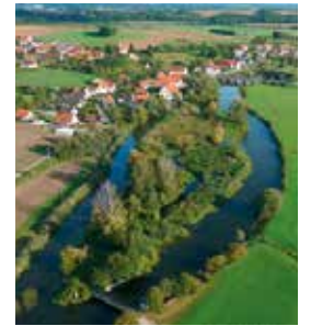
Wörnitz with millstream: Typical for the use of water power is splitting off into a millstream (waterway on left) and lower course. Water level is regulated by a low-head dam (in foreground).
